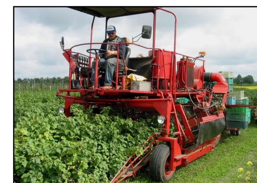
Fot. 3. Self-pulled "KPS 4b" harvester
